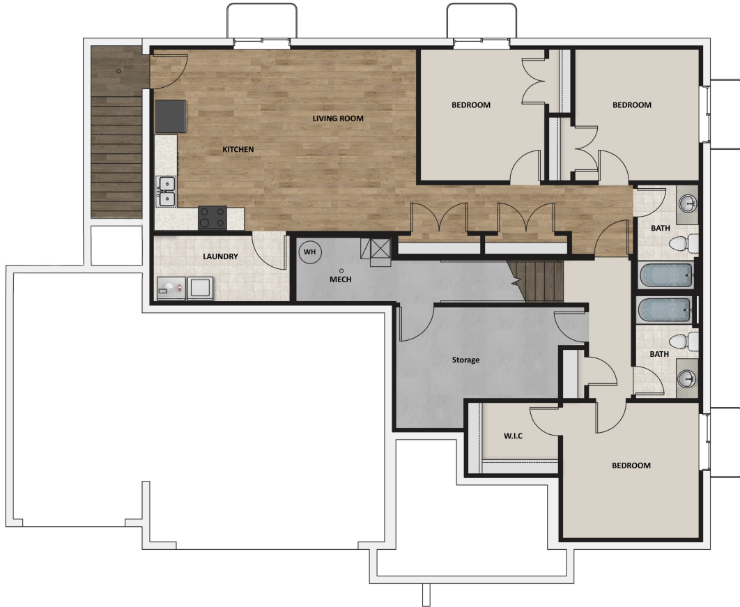
Finished Basement Floor
